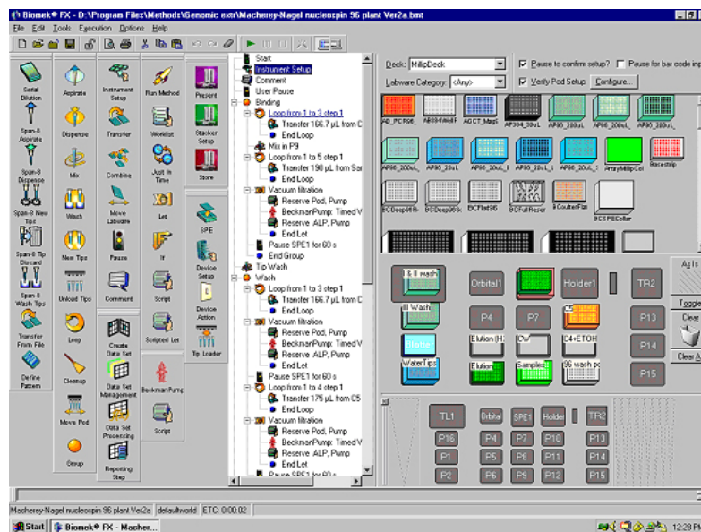
Fig. 2a) The genomic DNA extraction method on the Biomek FX platform
